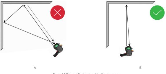
Figure 4.8 Do's and Don'ts when detecting the corner
