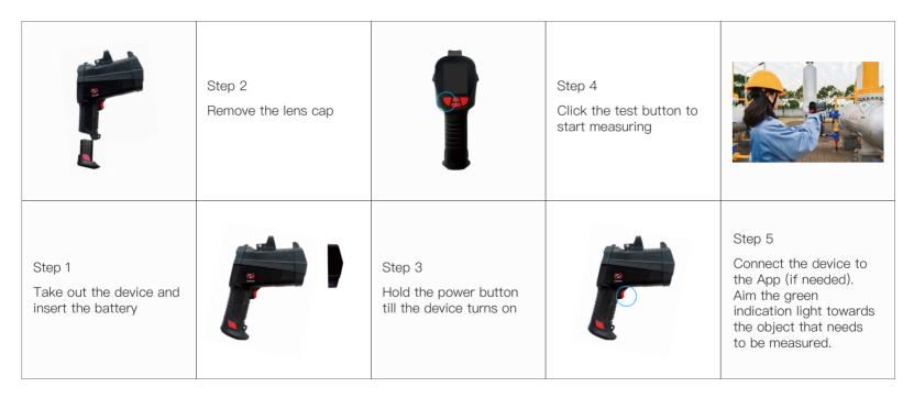
NOTE The red dot aiming sight, which is turned on once the device is powered on, can be used for better aiming.
