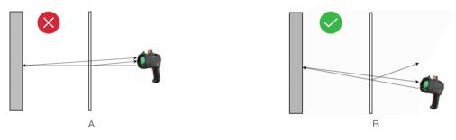
Figure 4.6 Do's and Don'ts when detecting through the glass
